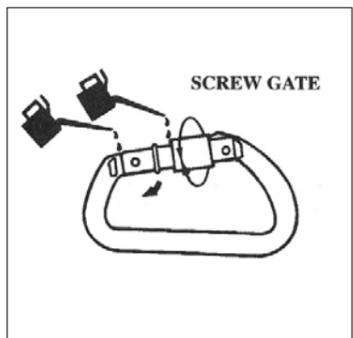
a) The karabiner gate hinge and screw or auto locking mechanism must be lubricated periodically and after any cleaning, drying or disinfect ion process to ensure smooth operation and corrosion resistance.
