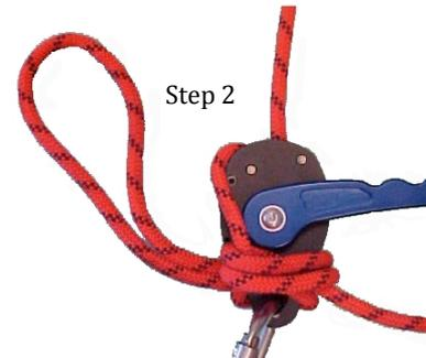
3. Finish with an overhand knot so that the bite of the rope is pointing towards the attachment point of the device.
