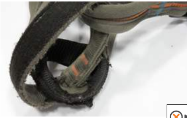
• Worn out belay loop and tie-in point
