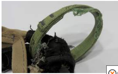
• Worn out belay loop and tie-in point
