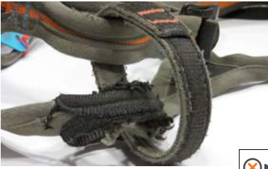
• Worn out tie-in point
