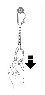
• Verify that the connector/sling/ STRING assembly is correct.
