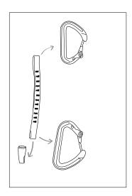
• Remove the connectors and the STRING from the quickdraw.
